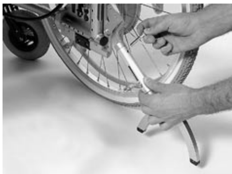
Fig. 27 Attaching the locking pin
