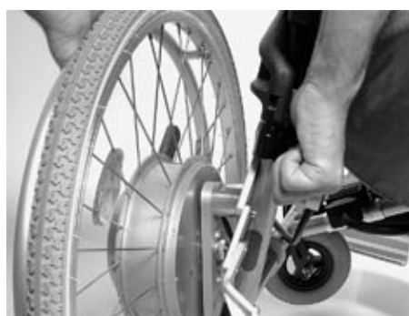
Fig. 8 Disassembling the z50 wheel
