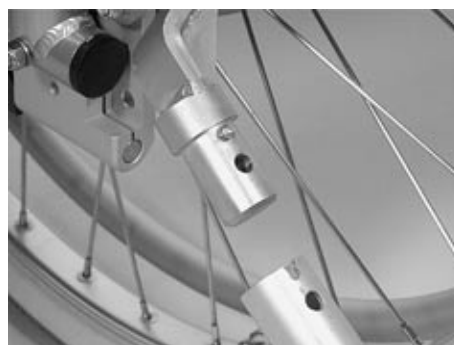
Fig. 26 Ratchet nose of the swinging anti-tipper
