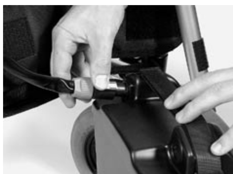
Fig. 15 Pulling off the battery cable
