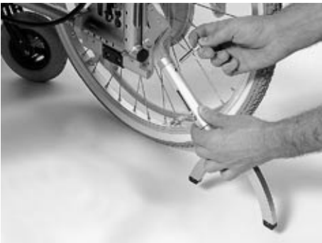
Fig. 23 Pulling off the swinging anti-tipper
