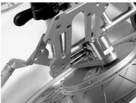
Fig. 4 Attach the attachment bolt into the receiver hook
