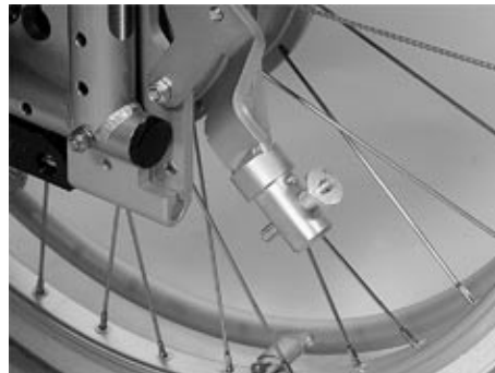
Fig. 24 Inserting the locking pin
