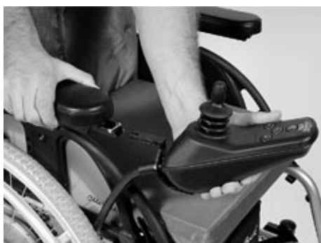
Fig. 16 Removing the control panel
