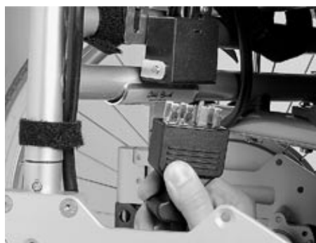
Fig. 17 Pulling off the central plug contact
